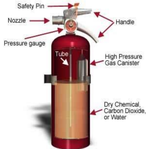
Fig 1.4: Basic fire extinguishers and its components.
